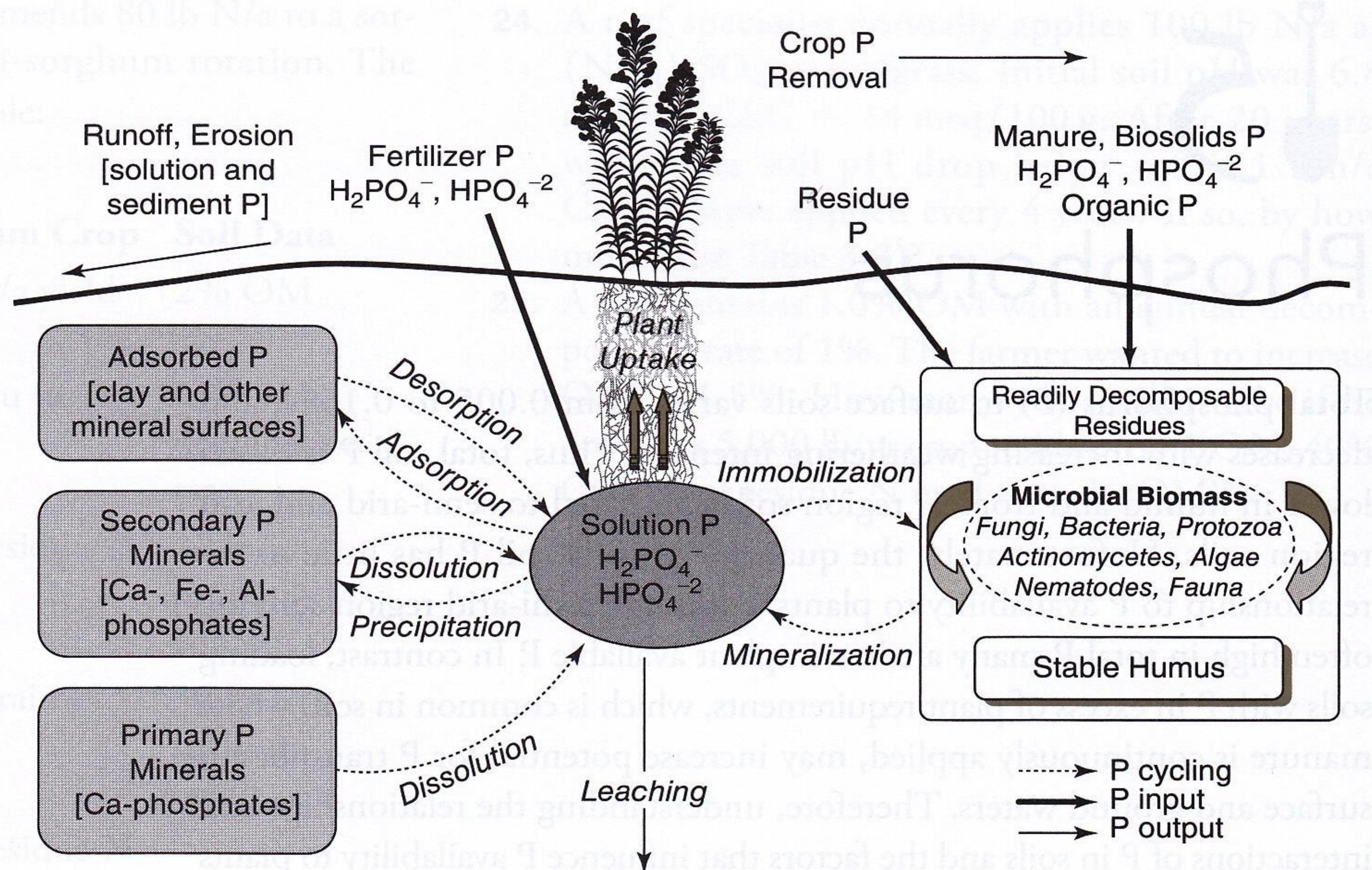
Internal P cycling between soil solution phosphorus and adsorbed P, solid mineral P, and organic P controls phosphorus availability to plants. Removal of phosphorus from the system occurs primarily through crop removal; however, phosphorus losses occur from soil erosion, runoff and leaching.
