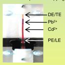
Dependence of the zone length on the dosing time (constant conc. of metal  $c= 2.10^{-5}$ ).
