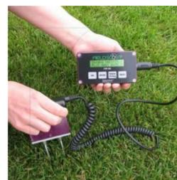
Fig. 7 Time domain reflectometry
