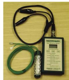
Fig. 4 Electrical-resistance device
