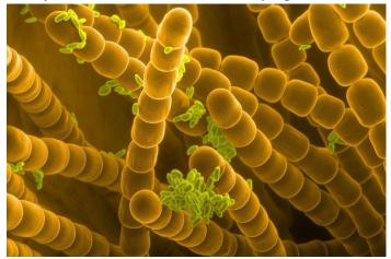
sample and generally does not add information about the specimen. In configurations some more information is gathered per pixel, often by the use of multiple detectors. The attributes of topography and material contrast can be obtained by a pair of backscattered electron detectors and such attributes can be superimposed on a single color image by assigning a different primary color each attribute. Similarly, to а combination of backscattered and
