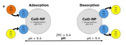
filter for field application. Xray diffraction and X-ray photoelectron spectroscopy experiments were used to examine adsorption, desorption, and readsorption of aqueous arsenite and arsenate by CuO-NP. Field experiments
