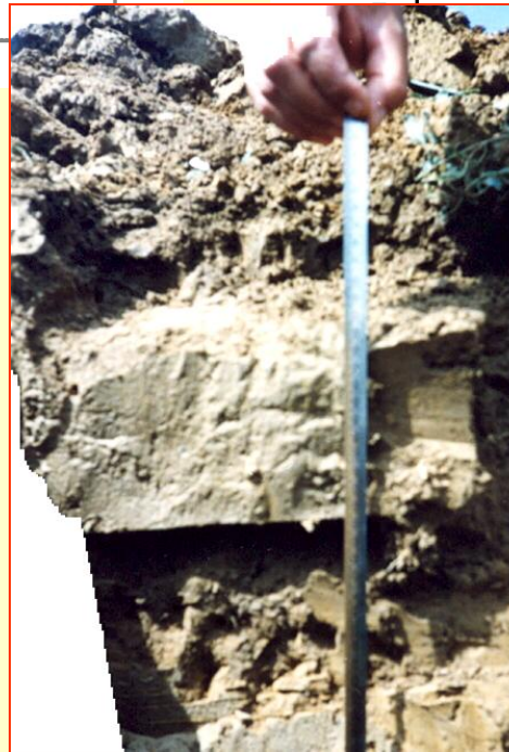
Soil in a loosened state and deteriorated by disk pan
