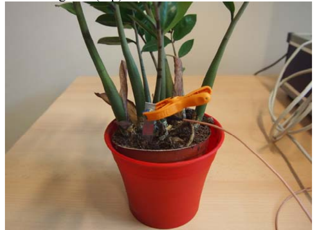
Fig.2 The position of an AE sensor installed on tip of AE waveguide (top)
