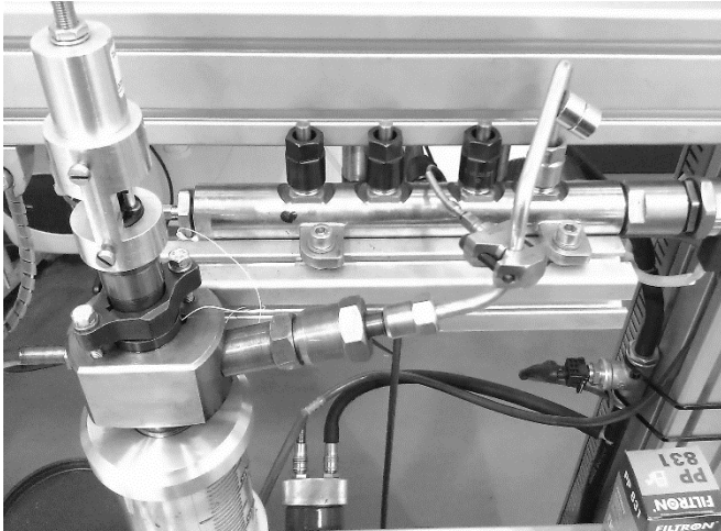
Fig. 2 Location of the piezoresistive pressure sensors at the test station
