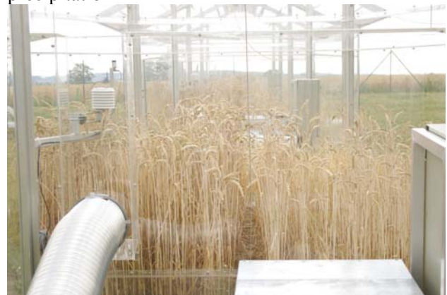
Fig. 1 Experimental site with 24 open-top chambers, which allows manipulation of [\text{CO}_2] and precipitation
