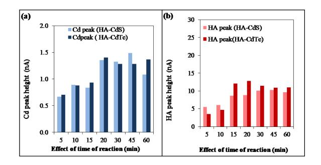
Optimization of time of reaction (binding HA-QDs complex to MPs modified by glycan). Effect of timeof reaction (min) was detected by electrochemical analysis of Cd peak (a) and HA peak (b). (a)Dependence of Cd peak height (nA) on time of reaction (min) and binding of HA-QDs on glycan. All measurements of Cd peak was used ASV DPV.
