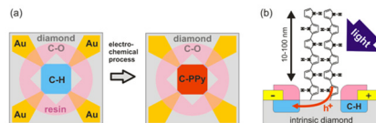
Figure 1.: (a) Diamond device for PPy synthesis and electronic transport measurements (b) Schematic cross-sectional view of PPy-diamond interface and effect of illumination.
