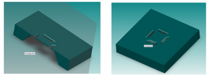
Figure 1.: Model of suspended membrane structure
