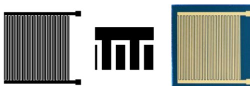
Figure 2.: Interdigital structure design, its detail and fabricated gold active layer electrode substrate
