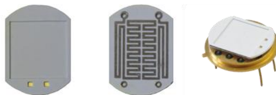
Figure 1.: The fabricated LTCC frame and its placement in TO-8 package
