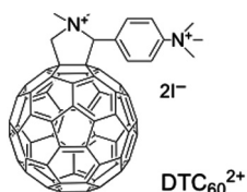
FIGURE 5.3 N,N -dimethyl-1-(2-(4-( N,N -trimethylaminophenyl)fulleropyrrolidinium iodide (DTC(60)(2+)) synthesized by 1,3-dipolar cycloaddition using 4-( N,N -dimethylamino) benzaldehyde, N -methylglycine, and fullerene C(60).
