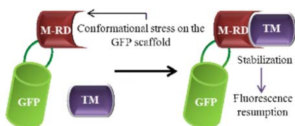
Fig. 3. Allosteric GFP-based biosensor. In the absence of the target molecule (TM), conformational influence of the molecular-recognition domain (M-RD) or receptor protein puts stress on GFP and thus reduces fluorescence yields. After binding with TM a stabilisation of conformation occurs resulting in a resumption of the GFP fluorescent ability.
