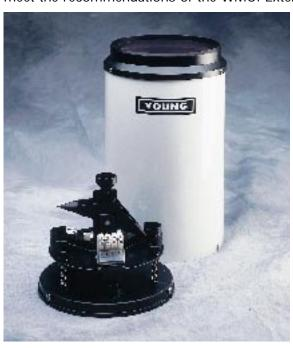
ensures maximum performance and value. Leveling screws and bullseye level are built-in for easy and precise adjustment in the field. Measured precipitation is discharged through a collection tube for verification of total rainfall. Model 52202 is heated for operation in cold temperatures. An unheated version, 52203, is available for use in moderate climates.
