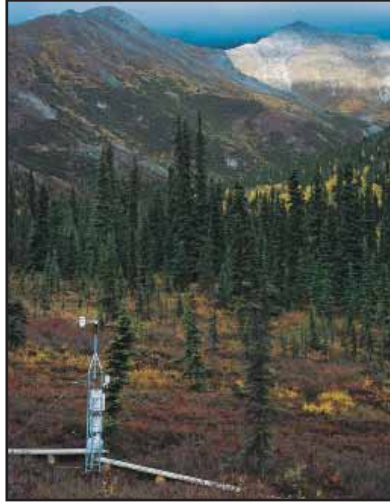
Weather station at Denali National Park, Alaska, monitors meteorological and soil conditions.
