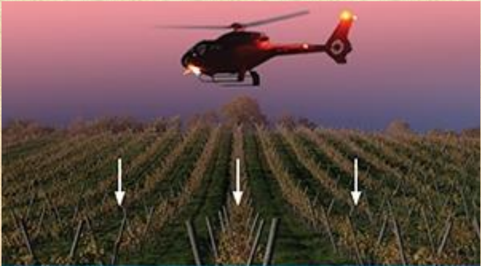
HELICOPTER FROST PROTECTION: Helicopter forces warmer air from inversion layer to ground level
